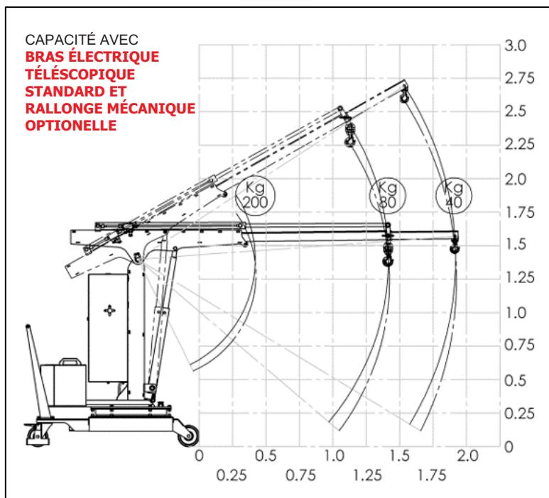
**SCP05M****Déplacement manuel****CARACTÉRISTIQUES PRINCIPALES****CAPACITÉ 500 KG****■ ÉLÉVATION MANUELLE**
