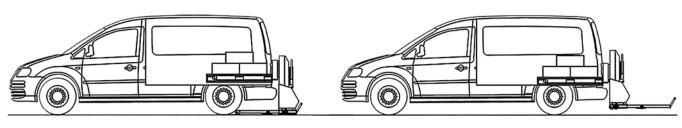
1 Pick up the load and lift the pallet
