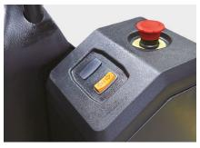
The tow truck is equipped with forward/reverse and up/down buttons on both sides. As a result, the operator does not need to get on and off the platform to operate the truck, improving picking efficiency and operational safety.
