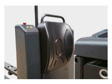
Safety flanks and non-slip surface materials on both sides of the backrest improve the operator's comfort and safety and reduce fatigue.
