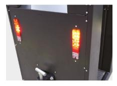
The directional light, brake light, and parking lights support safer driving.
