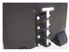
The reinforced hitches can be set to three different heights to ensure a reliable connection to diverse trailers.
