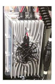
PSE12N SL stacker is equipped with a maintenance-free 24 V / 60 Ah **LifePO4** Li-ion battery. The fast-charge Li-ion battery has a large number of charge / discharge cycles. A 25 Ah charger is included.
