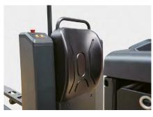
Safety flanks and non-slip surface materials on both sides of the backrest improve the operator's comfort and safety and reduce fatigue.
