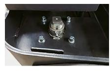
The upper fastening nut enables easy adjustment of the stabilizer wheel.
